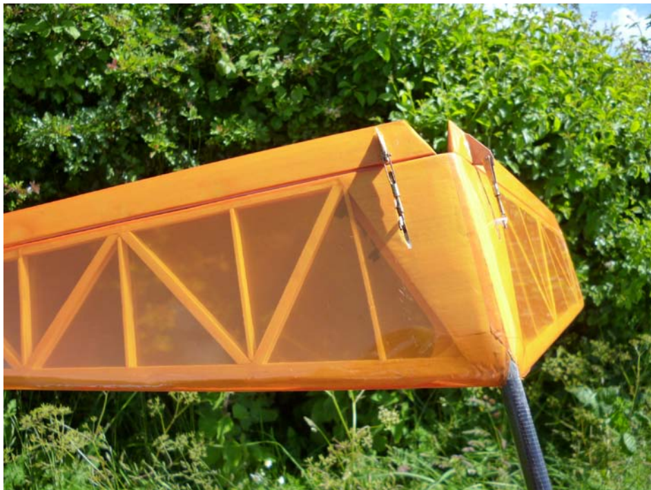
Neat tail and hidden servo detail on Jeff Fellows pusher design.
